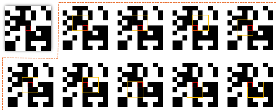
Figure 6. Illustration for the stitching. For the 3x3 block configuration setting, each target location (red box) is covered by nine overlapping block images (yellow box).
